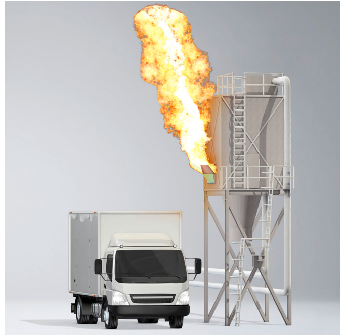
With TARGO-VENT: The flame is deflected into safe areas.
